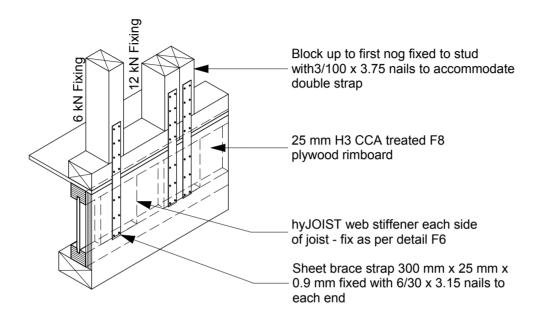
**Detail TD1** Tiedown for external bracing wall using rimboard **6 & 12 kN fixing details** Scale: NTS May 2007
