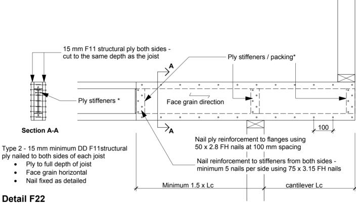
Cantilever supporting load bearing walls- Type 2 reinforcement May 2007
